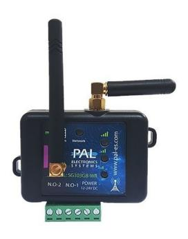
Modules for remote access control for barriers, gates or turnstiles by mobile phones or remote controls.
